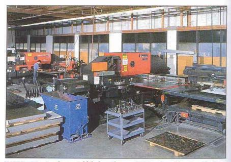
MASS Precision is a sheet metal fab shop. They use CNC turret punch presses, like these from Amada, to fabricate parts for electronic cabinetry. Equipped with load/unload stations, the presses help increase throughput by keeping work "in the cut."
